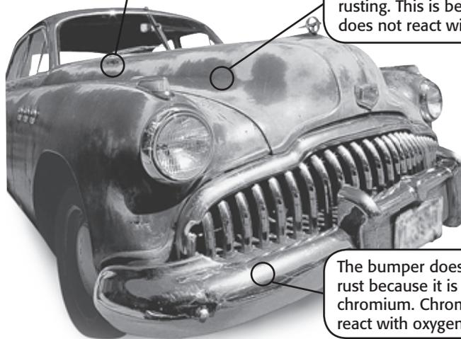
The bumper does not have any rust because it is covered with chromium. Chromium does not react with oxygen.
